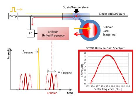
The NEUBRESCOPE NBX-5101 is single-ended Brillouin OTDR for fiberoptic distributed Strain and Temperature measurement.
