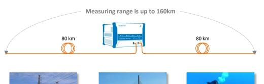
By the setting and the operation of the Sequence Mode in the NEUBRESCOPE software, the measurement results from two fibers can be kept. It gives the total distance up to 160km.
