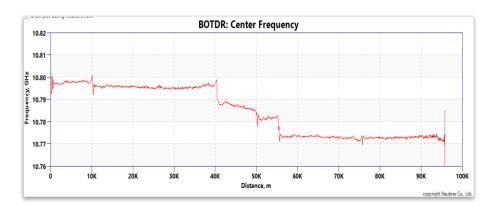
The NBX-5101 is capable to measure the distance up to 80km either by Brillouin OTDR or by Coherence OTDR.
